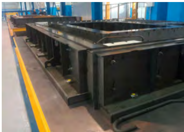
SAS-MF in solid wall production
