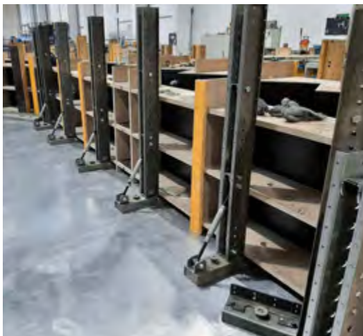
Easy Form with vertical supports can be used to create bar-shaped elements or, e.g. stairs
