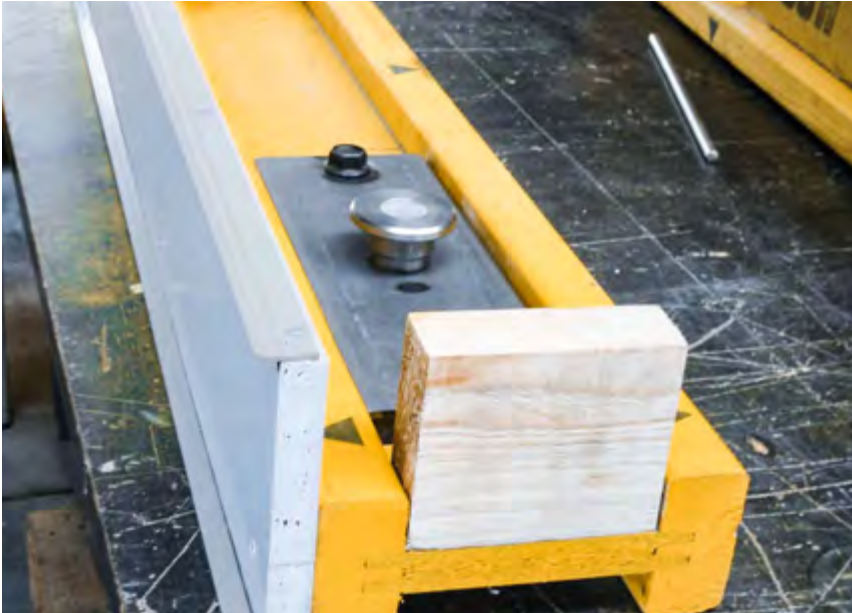
SPB with Doka plywood beam
