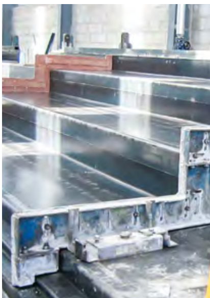
SPB for fixing staircase moulds
