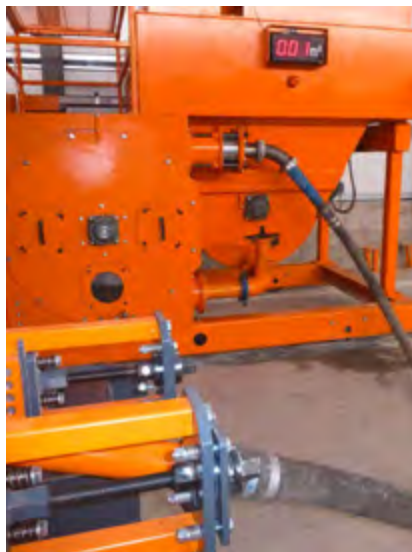
Concrete filling connection UCI Square
