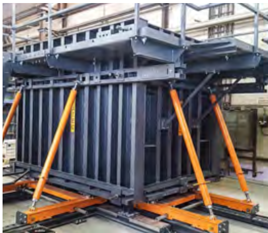
Example: Shuttering for the production of transformer stations measuring 2.4 x 2.1 x 2.3 m and 2.9 x 2.1 x 2.3 m
