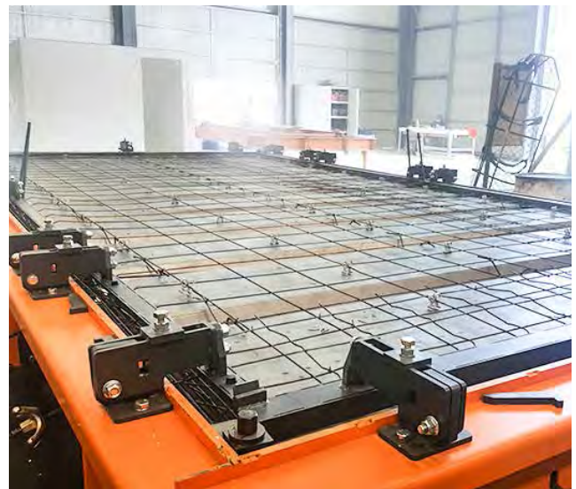
Moulds for a flat roof with contouring at the bottom for filling from above
