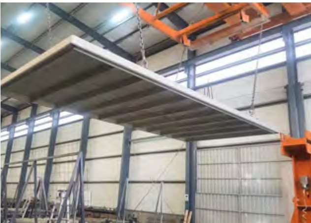
Example: Roof moulds for upcrete®, filling from below
